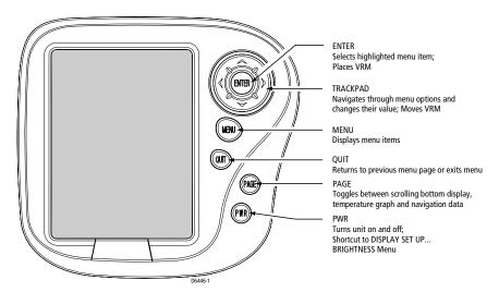
Figure 3-3: Keypad Functions
